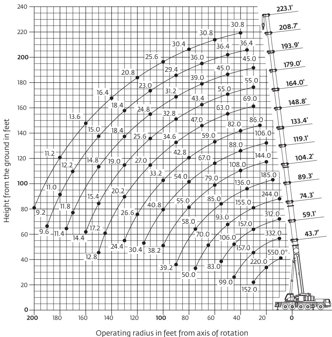
*Hook heights shown in the working diagram do not consider loaded boom deflection.*
