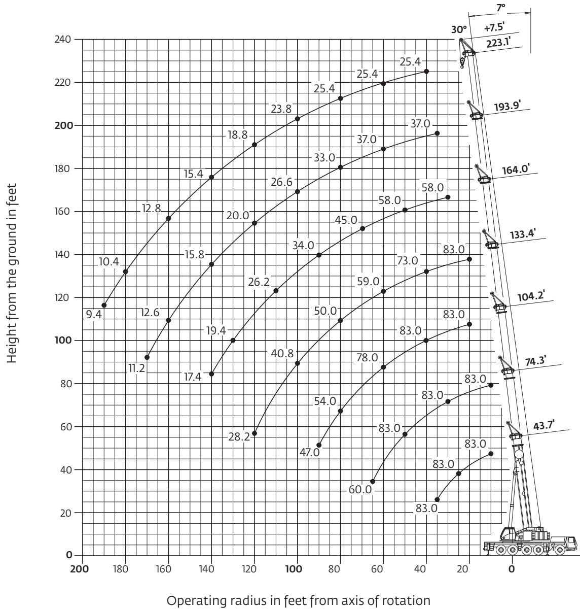
Hook heights shown in the working diagram do not consider loaded boom deflection.
